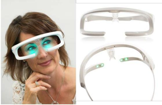
Picture 1: Re-Timer device utilizing 500nm wavelength
